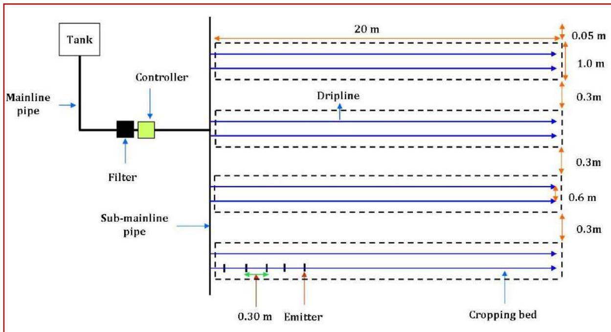
Figure 4: Drip irrigation system layout for 20x5 m greenhouse
