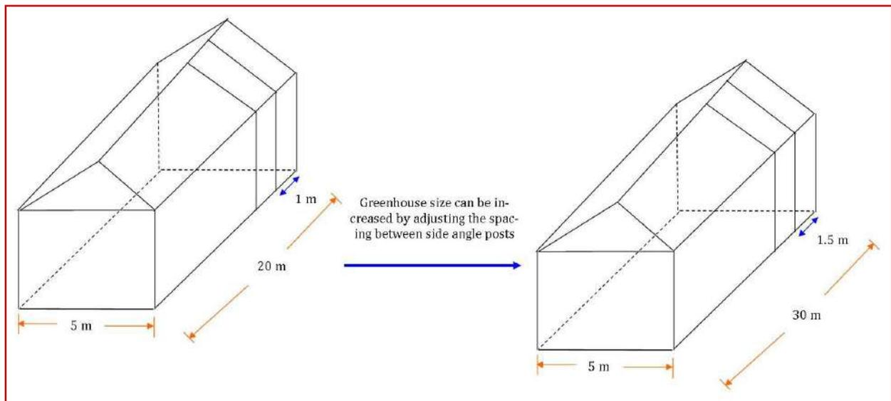
**Figure 3:** Increasing the size of 5x20 m greenhouse
