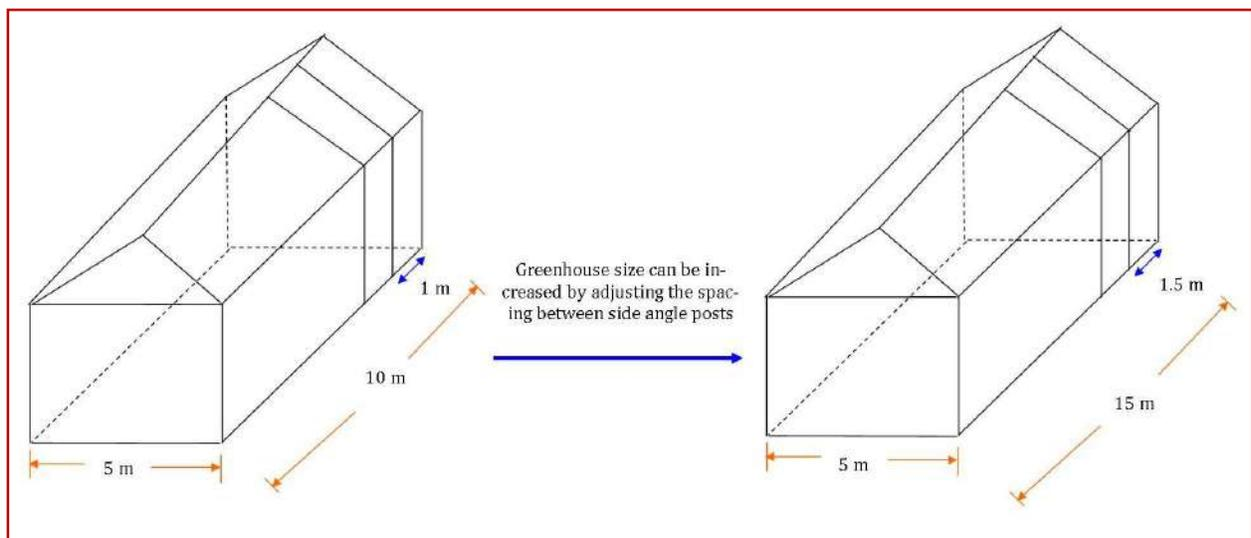
**Figure 2:** Increasing the size of 5x10 m greenhouse
